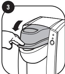
3 Lower the Handle completely and firmly to close the Lid and puncture the K-Cup® portion pack.
